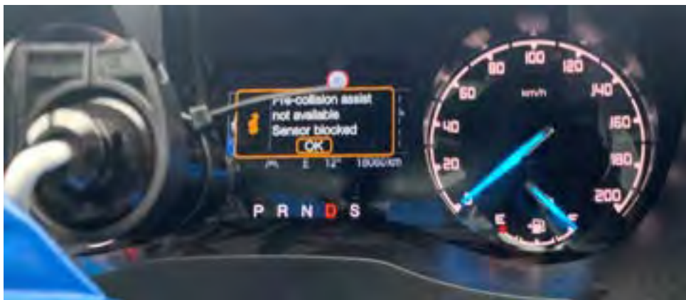
Figure 78: Ranger sensor blocked warning that was observed during testing.
