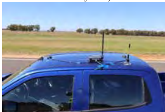
GPS Antennas mounted to vehicle roof
