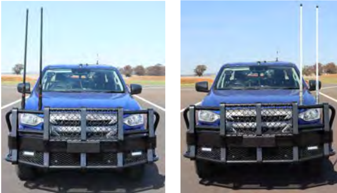
Figure 21: Antennas mounted to the Isuzu D-Max: Dual black Antennas on the driver's side (Left) and dual white Antennas on the passenger side (Right).
