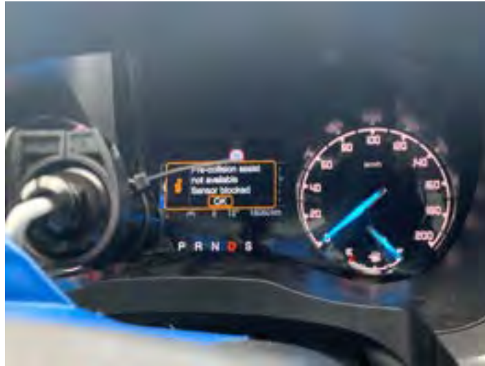
Figure 72: Ford Ranger sensor blocked warning.
