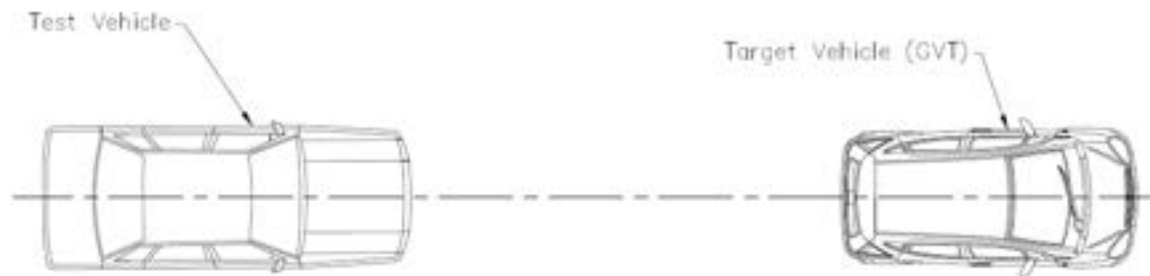
Figure 9: Car-to-Car testing scenario with test vehicle approaching target vehicle from behind.
