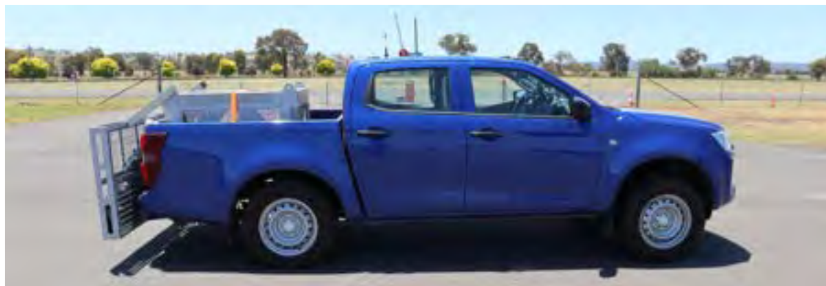
Figure 23: Isuzu D-Max in the worst-case rear pitch load configuration.
