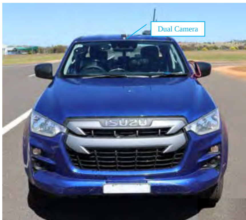
Figure 18: Isuzu D-Max dual camera system location.
