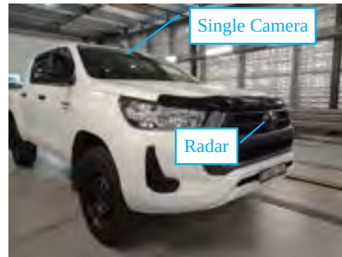
2020 Toyota Hilux Camera and Radar Location
