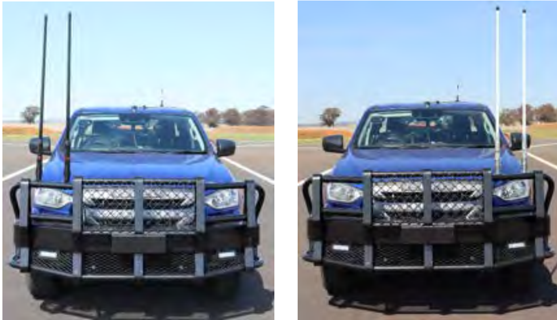
Figure 7: Antennas mounted to the Isuzu D-Max: Dual black Antennas on the driver's side (Left) and dual white Antennas on the passenger side (Right).
