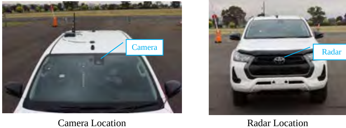
Figure 17: Toyota Hilux camera location (left) and radar (right) location.
